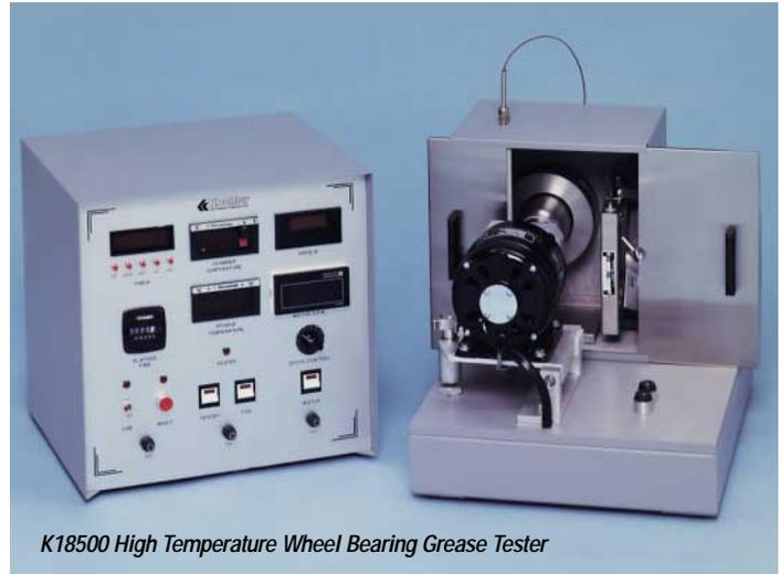
K18500 High Temperature Wheel Bearing Grease Tester
