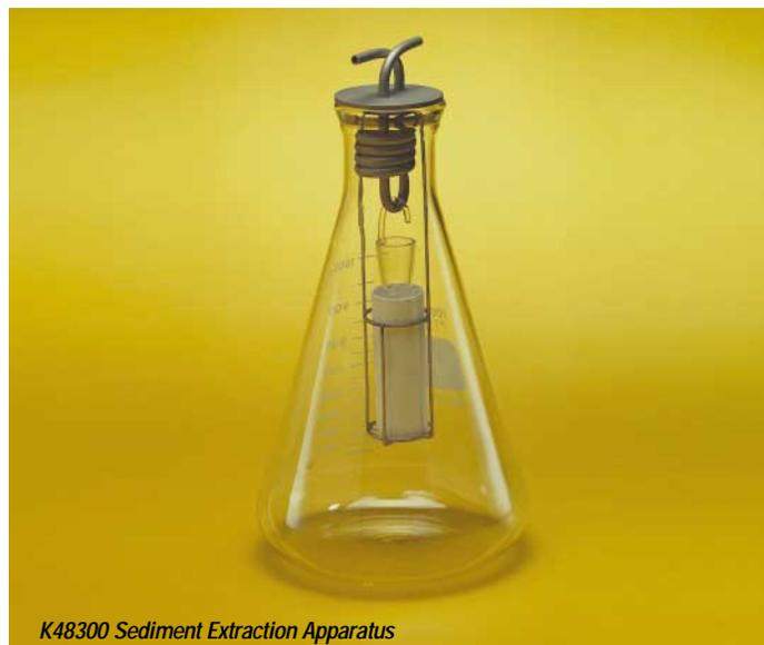
K48300 Sediment Extraction Apparatus
