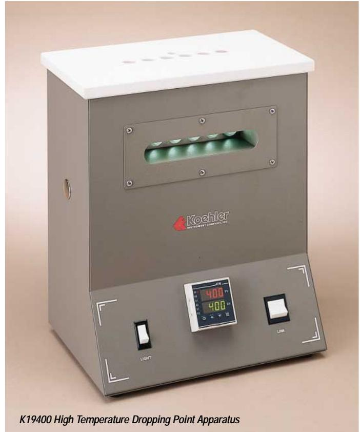
K19400 High Temperature Dropping Point Apparatus
