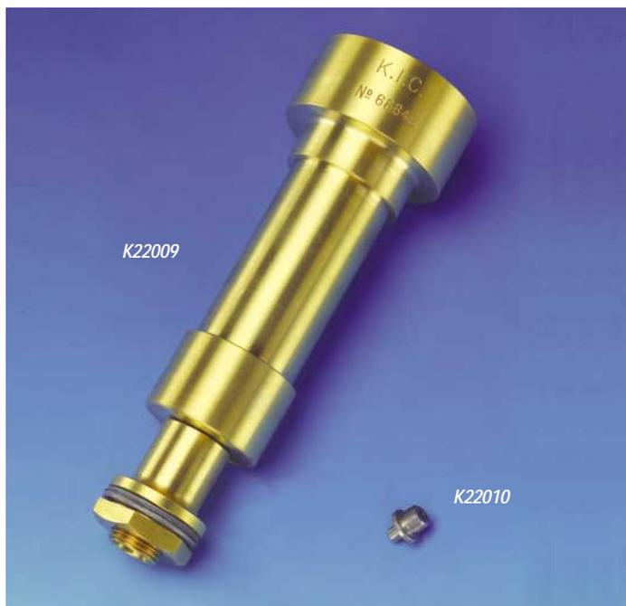
**Orifices**—Stainless Steel Universal and Furol Orifices meeting ASTM specifications. Orifices insert in viscometer tubes using K22030 Orifice Wrench (supplied with viscometer baths). Also available - Kansas Road Oil Orifice (requires K22039 wrench). Universal and Furol Orifices are available with a calibration certificate.
