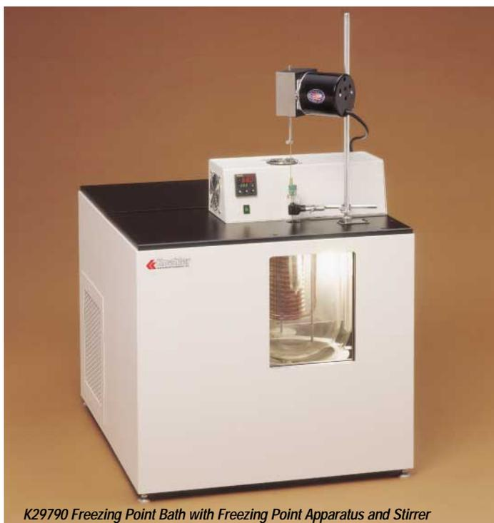
K29790 Freezing Point Bath with Freezing Point Apparatus and Stirrer
