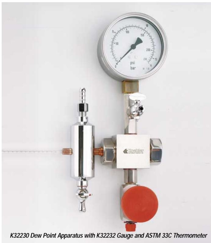
K32230 Dew Point Apparatus with K32232 Gauge and ASTM 33C Thermometer
