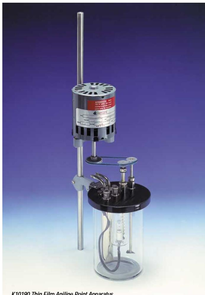
K10190 Thin Film Aniline Point Apparatus
